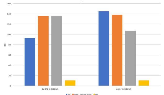
Fig. 12. Comparison of latency during and after the lockdown, RTT is in milliseconds.
