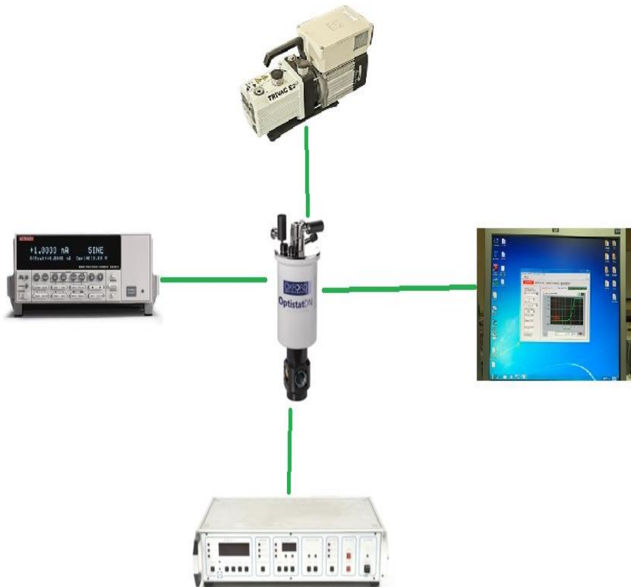
Figure 3 - IV experiment setup schematic diagram showing the main equipment used to detect the IV characters of the QD LD
