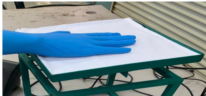
Fig. 3. Gloves sliding against textile specimens.
