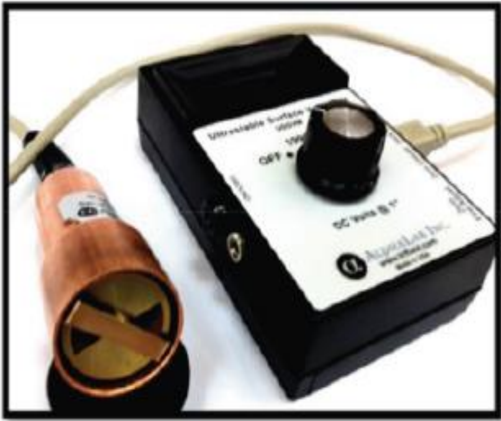
Fig. 1 Electrostatic charge (voltage) measuring device.
