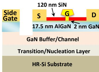
Fig. 1: Schematic diagram of the AlGaN/GaN HEMT with side gate on a high resistivity silicon substrate
