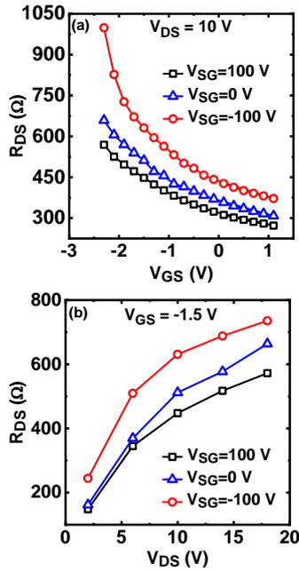
Fig. 9: Extracted  $R_{DS}$  versus (a)  $V_{GS}$  and (b)  $V_{DS}$  at three different  $V_{SG}$ .
