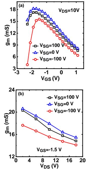
Fig. 4: Extracted intrinsic  $g_m$  versus (a)  $V_{GS}$  and (b)  $V_{DS}$  at three different  $V_{SG}$
