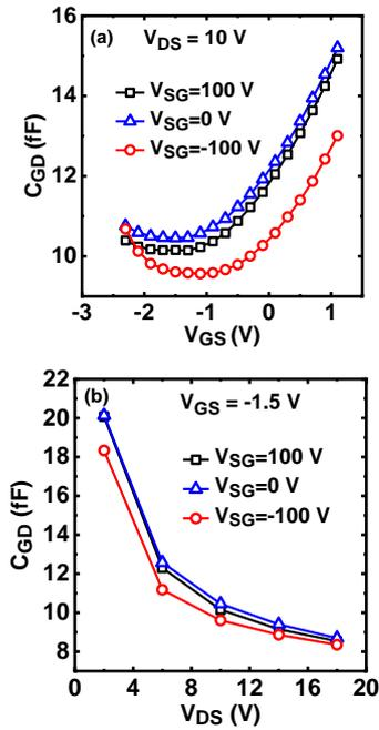
Fig. 6: Extracted  $C_{GD}$  versus (a)  $V_{GS}$  and (b)  $V_{DS}$  at three different  $V_{SG}$ .
