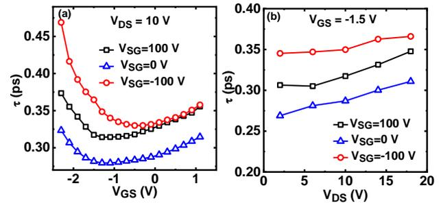
Fig. 11: Extracted intrinsic time constant  $\tau$  versus (a)  $V_{GS}$  and (b)  $V_{DS}$  at three different  $V_{SG}$ .
