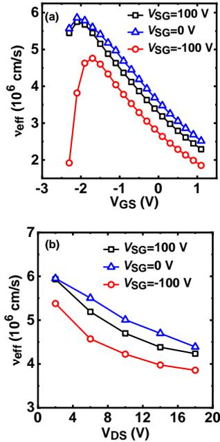
Fig. 8: Calculated  $v_{\text{eff}}$  versus (a)  $V_{\text{GS}}$  and (b)  $V_{\text{DS}}$  at three different  $V_{\text{SG}}$ .
