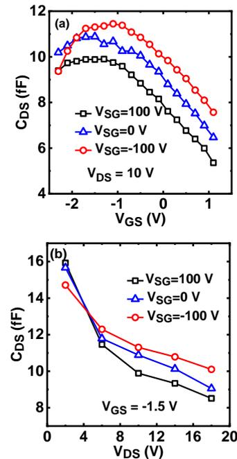
Fig. 7: Extracted  $C_{DS}$  as a function of the (a)  $V_{GS}$  and, (b)  $V_{DS}$  at three different  $V_{SG}$
