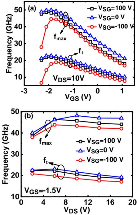
Fig. 2: Measured  $f_t$  and  $f_{max}$  values versus (a)  $V_{GS}$  and (b)  $V_{DS}$  at three different  $V_{SG}$ .
