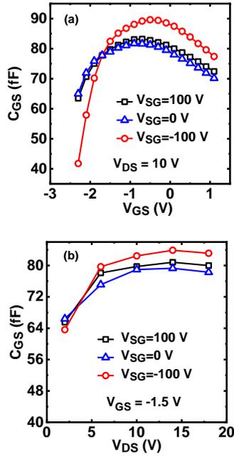
Fig. 5: Extracted  $C_{GS}$  versus (a)  $V_{GS}$  and (b)  $V_{DS}$  at three different  $V_{SG}$ .
