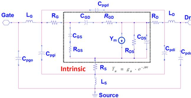
Fig. 3: Schematic of a small-signal equivalent circuit [15].
