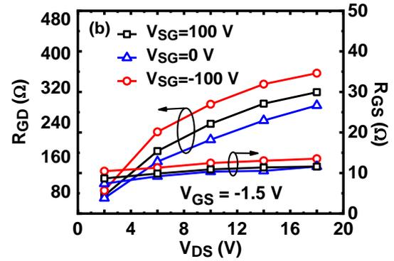
Fig. 10: Extracted  $R_{GD}$  and  $R_{GS}$  versus (a)  $V_{GS}$  and (b)  $V_{DS}$  at three different  $V_{SG}$ .
