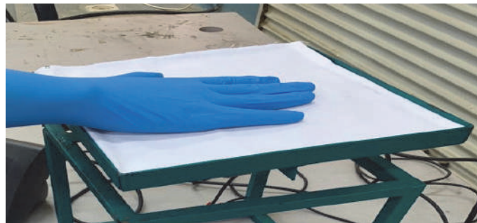
Fig. 3. Gloves sliding against textile specimens.
