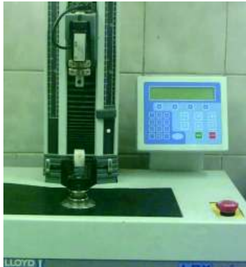
Fig. 3. The Lloyd Universal Testing Machine and the mounted specimen during shear bond strength testing.
